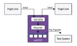
Record the flight hardware's XAUI output to RAID5 disk storage/ network storage. Using the XAUI loopback feature creates a "T" in the data flow to capture hardware-to-hardware data transfers. Transfer recorded files for analysis or archive.
